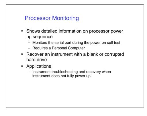
Power Up Monitoring is a technique that can be used to diagnose turn on problems or errors with the 8960. There are three types of monitoring; Host Processor Logging, DSP Processor Logging, and Protocol Processor Logging.
